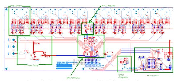
Figure 5: Sabre DAC Reference 64LQFP Evaluation Board
