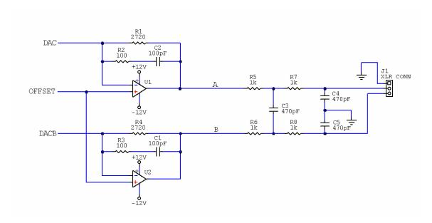
Figure 1: Sabre Reference Evaluation Board Differential Output
