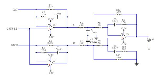
Figure 2: Sabre Reference Evaluation Board Single Ended Output
