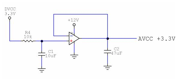
Figure 4: AVCC +3.3V Filter and Regulator
