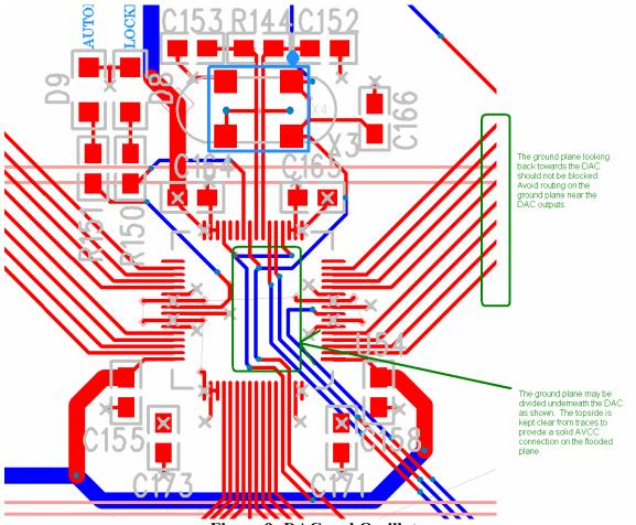
Figure 9: DAC and Oscillator
